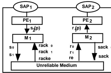
**Figure 18.** Alternating bit for an unreliable medium
